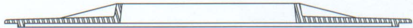
EXTENSION RING ALLOWS INSTALLATION OF STANDARD FRAME AND COVER ON 24" THRU 36" METER PIT
