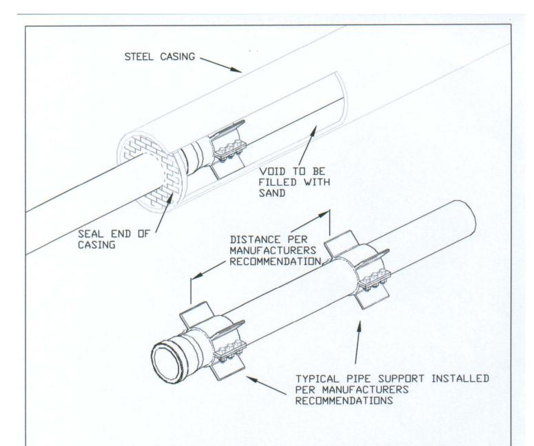
DIAMETER OF CASING SHALL BE DETERMINED BY THE ENGINEER.
