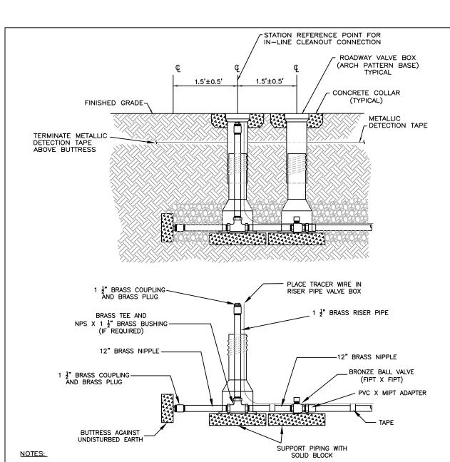
BLOCKING SHALL BE SOLID BLOCK OR CONCRETE.
